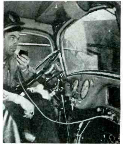
Operating simplicity is a prime feature of f-m installation in truck freighter. Designed by Motorola, the transceivers have been tested in trucks of Standard Freight Lines
