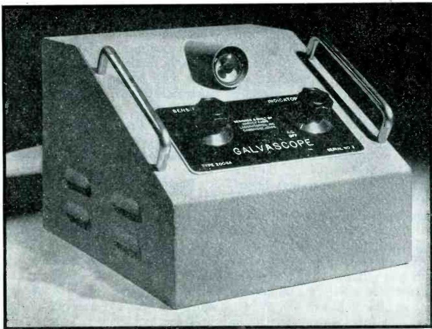
Exterior of the electronic a-c galvanometer, showing hooded indicator tube and operating controls. The indicator bias knob at the right has an associated on-off switch for 115-v, 60-cycle a-c power. Tubes and other components are accessible after removal of bottom plate
