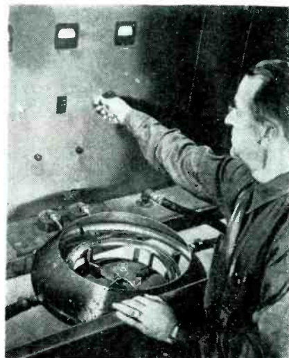
Flywheel ring gear for a Studebaker is set up in the hardening fixture recently added to the production line. With this equipment, a better gear is produced with a 99.9 percent reduction in heat-treating time
