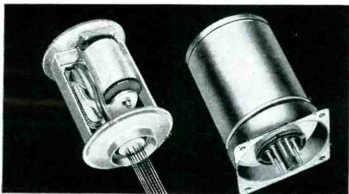
Larger relay, with specially designed anchor plate mounting to withstand shock and vibration up to 20Gs. Relay is bolted to heavy bracket and anchor plate (top left) and base plate. Completed enclosure (right) shows beads rolled into top and bottom of housing to grip both plates, and square base for bolting to frame. Lead wires have been soldered to octal plug.
