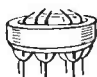
Headers —The best way to get a large number of leads in a small space for assembly in one operation.
